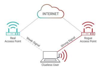
Figure 5: Diagram of a compromised access point
